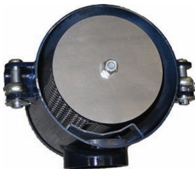
Inlet Filter with lid removed
